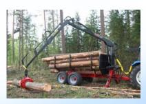
Trailer application including floating of the boom and traction
